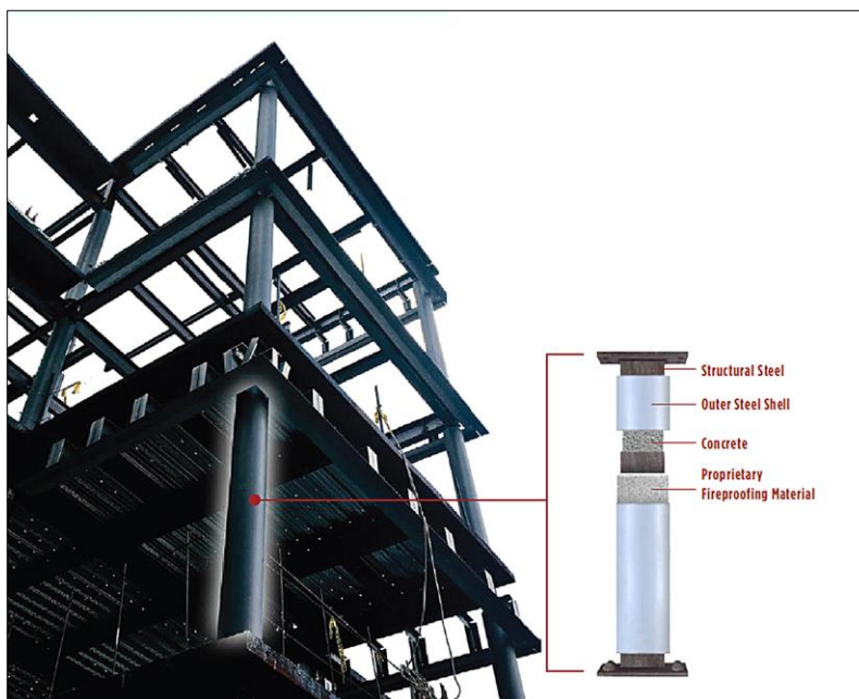
Fire-Trol® fireproof column description (Photo courtesy of Fire-Trol®)
